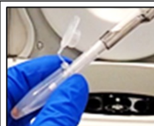
Figure 5: Using the tip of a pipette, carefully remove all of the remaining Wash Buffer that has collected just below the magnetic bead pellet.
