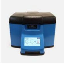
The Bullet Blender Gold<sup>+</sup> combines 4°C Cooling<sup>™</sup>, noise insulation to keep homogenization quiet, and an extra-powerful motor for tough samples. This homogenizer is ideal for tissue or cell cultures. It can process up to 24 samples in parallel, homogenizing up to 300 mg of sample in each microcentrifuge tube.
