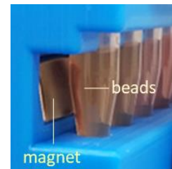
Figure 2: Magnetic beads separate to the back wall of the tubes, when placed in the magnetic rack.
