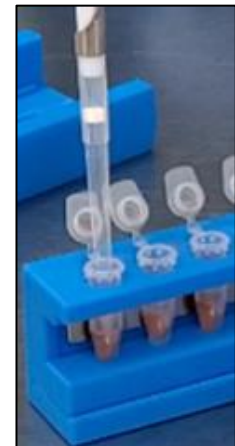
Figure 3: Using pipette tips, carefully remove the supernatant. If needed, hold the tube to prevent the tube from moving/spinning.
